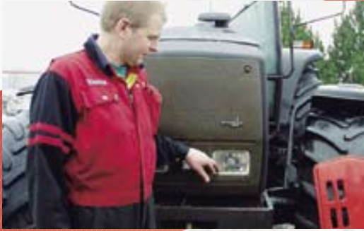
Danish farmer Peter Siig's Valtra 8750 has suffered a broken headlamp and front mask during heavy work. The tractor should be put into working order as fast as possible.
