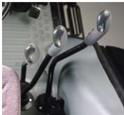
Gear levers from right-to-left: forward/reverse shuttle, four-speed main gear selector, and selector for intermediate ratios.
