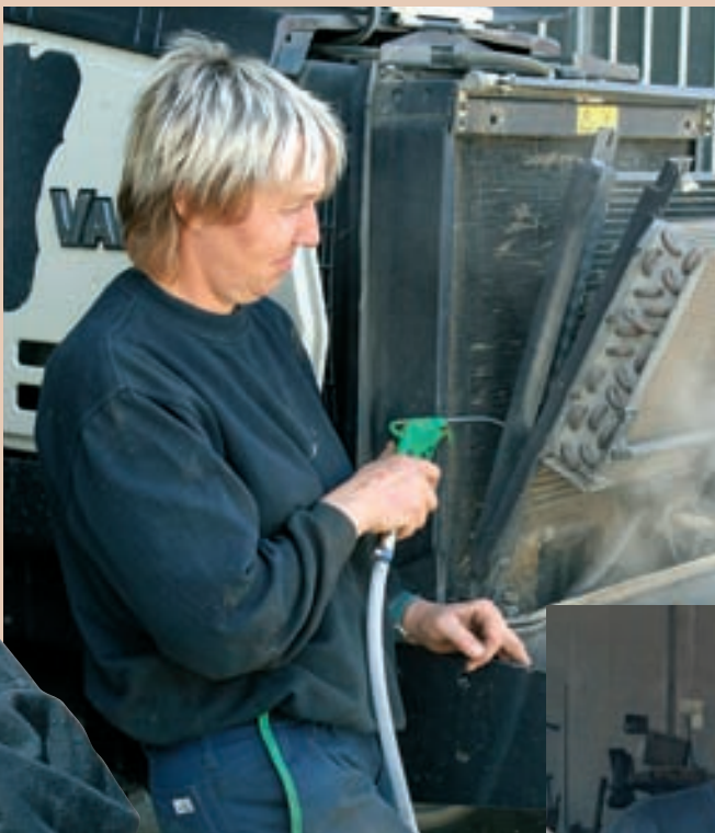
▲ The radiators may need to be blown clean after driving in dusty conditions. It is a good thing that they are so accessible.
