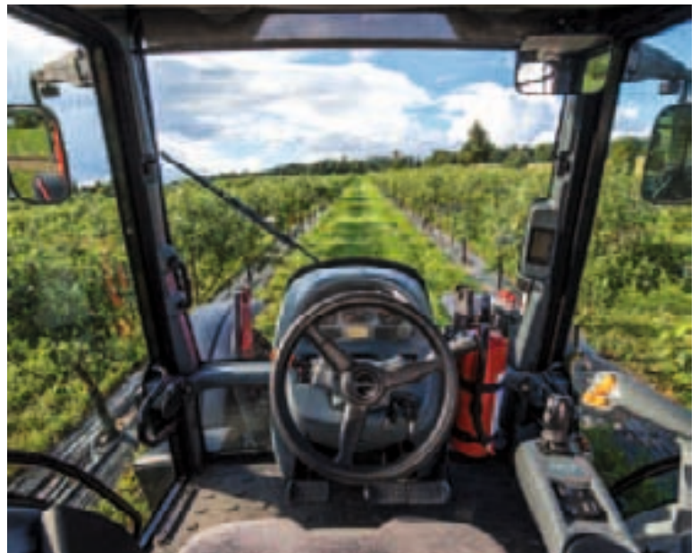
Visibility from the cab is excellent thanks to lowered cooling-package.
