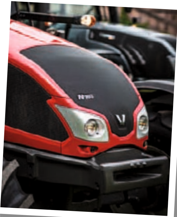
The nose has a new look: The new H7 bi-halogen lights combine both full and low beams.
